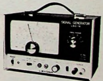
LSG-16 TOONGENERATOR 120 kHz-300 MHz
